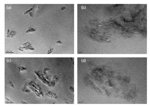
Fig. 5. TEM images of (a and b) PP74/WF20/MAPP3/clay3(with ballmilling); (c and d) PP54/WF40/MAPP3/clay3(with ballmilling) composite. Scalebars of (a and c) and (b and d) are 200 and 20nm, respectively.
