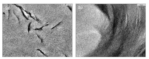
Fig. 3. TEM images of PP97/clay(3 wt.%) composite. Scalebar of (a) and (b) is 200 and 20nm.
