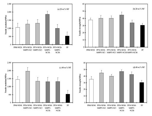
Fig. 1. Tensile modulus (a and c) and strength of (b and d) of PP/WF/MAPP/clay composites.
