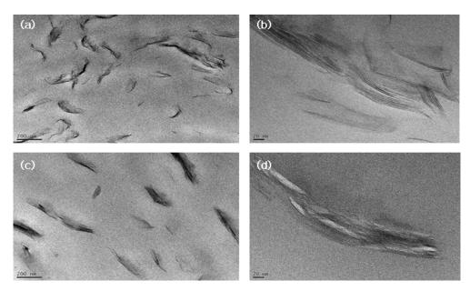
Fig. 4. TEM images of (a and b) PP74/WF20/MAPP3/clay3(without ballmilling); (c and d) PP54/WF40/MAPP3/clay3(without ballmilling) composite. Scalebars of (a and c) and (b and d) are 200 and 20nm, respectively.
