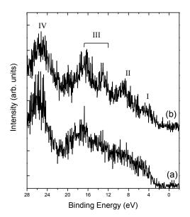
Fig. 7. The valence band (VB) spectra of (a) BZ-polyamide-acid film after curing at 150 °C for 1 hour and (b) BZ-polyamide-imide film after curing at 250 °C for 3 hours.
