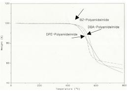
Fig. 3. TGA thermograms for polyamideimides
