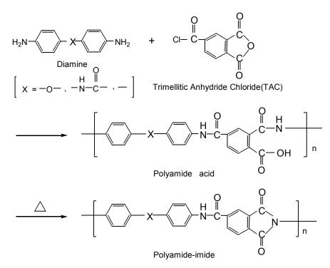
Fig. 1. Polymerization Scheme
