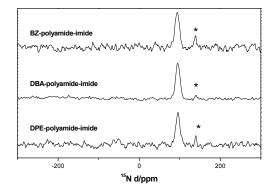
Fig. 6. NMR data for polyamide-imides after curing at 250 °C for 3 hours.
