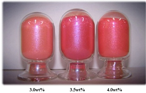
Fig. 3. Photographs of carmine coated mica with various amount of carmine for control pH.
