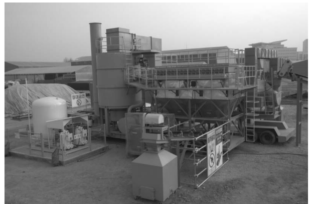
Fig. 6. Field application of LTTD for hydrocarbon-contaminated soil.
