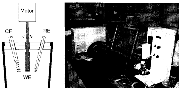
Fig. 1 RDE cell stand consisting of three electrodes (left, CE: counter electrode, WE: working electrode, RE: reference electrode) and voltammetric analyzer system (right).
