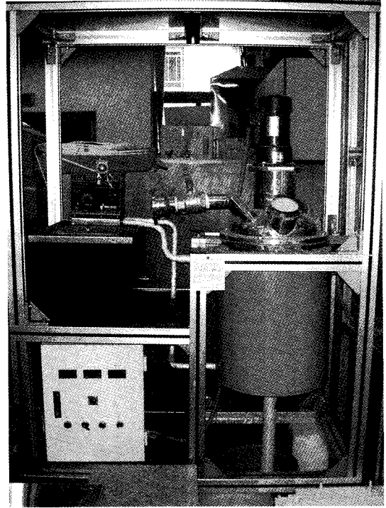
Fig. 3. The apparatus of hydrothermal synthesis for the bench scale.
