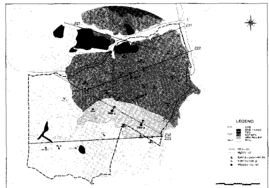
Fig. 2. Geological map around LILW repository site and location map of boreholes around LILW repository site; KB series well field and DB-series well field
