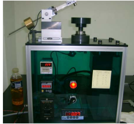
Fig. 2 Reciprocation wear testing system
