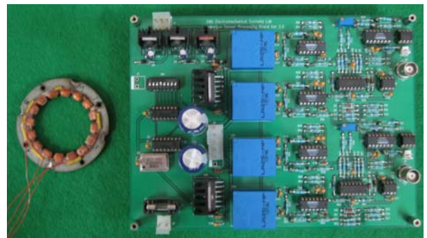
Fig. 4 Inductive position sensor and sensor signal processing circuit
