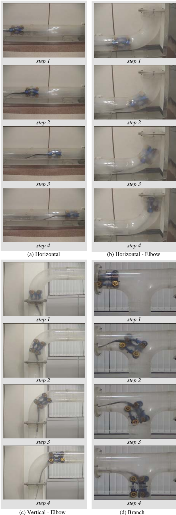
Fig. 12 Driving test in pipeline
