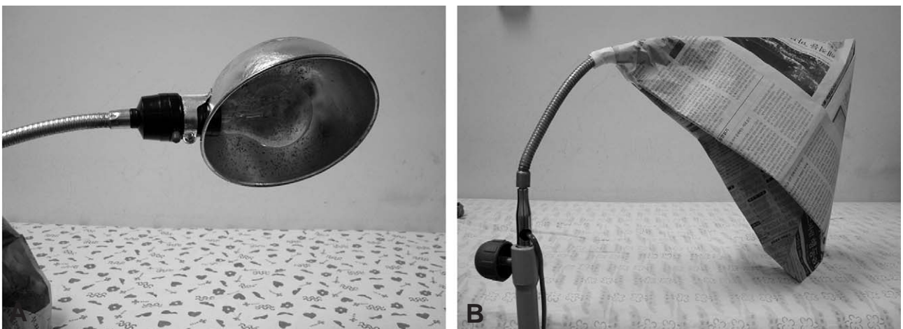
Fig. 1. Existing heat lamp (A) General light stands having 60 watt light bulb of incandescence and lampshade made of aluminum. (B) Covered with newspaper.
