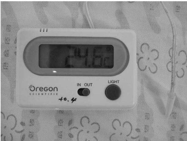
Fig. 3. Thermometer (range: -5~50℃, AW, Oregon Scientific)
