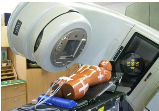
Fig. 3. Tangential irradiation and measurements set-up using MOSFET detectors on the humanoid Rando phantom.
