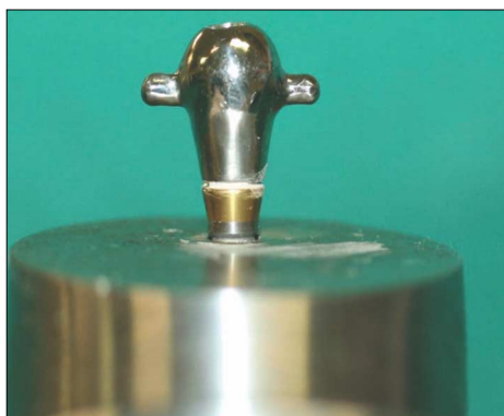
Fig. 1. The specially customized metal cap; hemisphere shape in order to transmit the applied load to the center of abutment.
