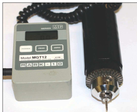
Fig. 2. Digital torque gauge (MGT12.mark-10. corp. USA). All abutment screws were tightened to 30 N/cm \pm 0.5 N/cm with this digital torque gauge and the removal torque values of the screws were recorded.
