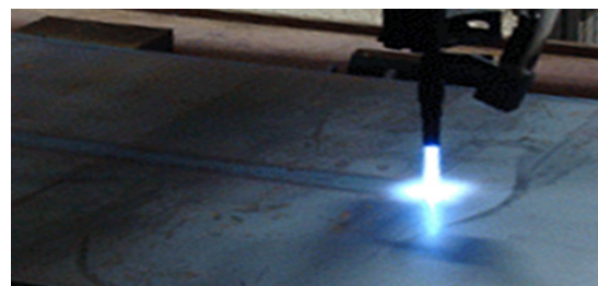
Fig. 3 Photograph of line heating
