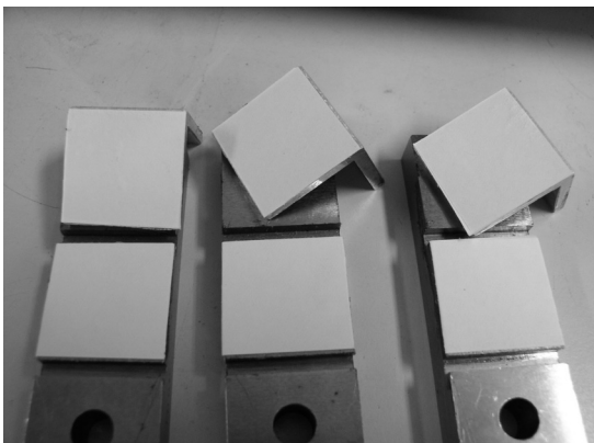
Fig. 3. Rupture at the adhesion area.
