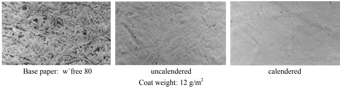
Fig. 1. SEM photomicrographs of woodfree base paper, and coated paper before and after calendaring.
