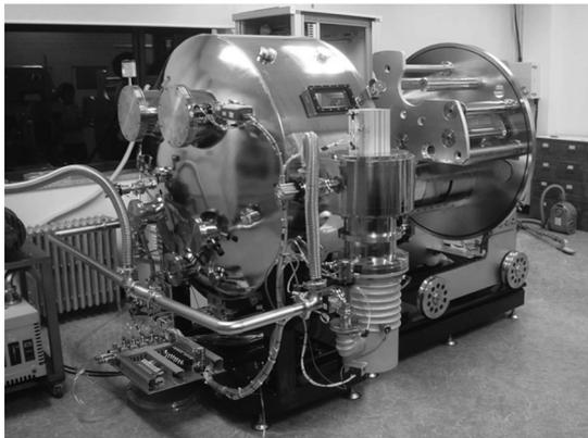
Fig. 1. Schematic diagram of Roll-to-Roll sputter system and picture.
