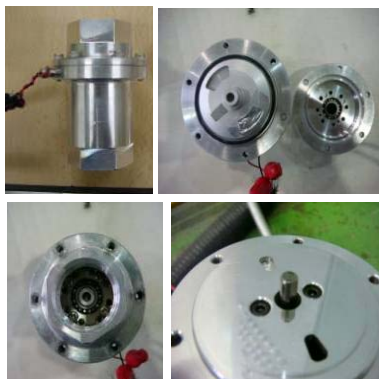
Fig. 2 Cyclic oscillating control valve
