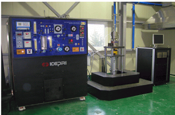
Fig. 5 Low-cycle environmental fatigue test rig
