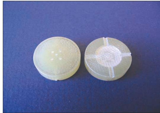
Fig. 3. Micro-channels, lateral channels and central well were prepared for water pumping effect.
