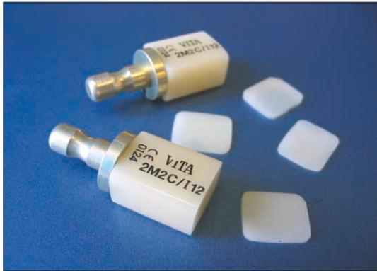
Fig. 2. Specimens were sectioned from Mark II blocks.
