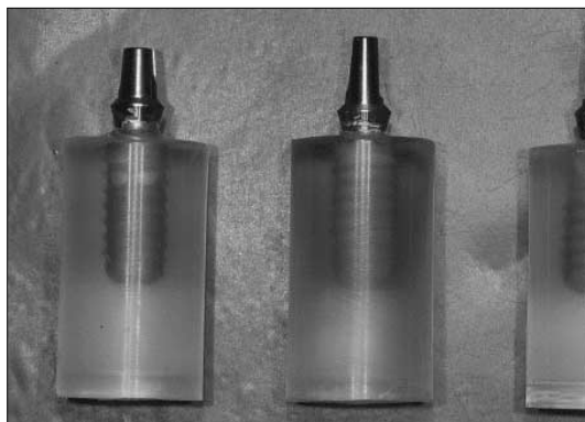
Fig. 1. The single implant with the solid abutment embedded in the block of acrylic resin.
