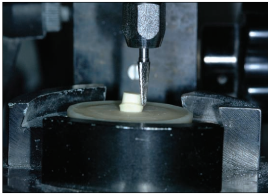
Fig. 1. Preparation of resin tooth by using milling machine.
