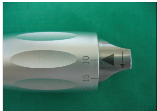
Fig. 6. 10Ncm setting of torque controller.
