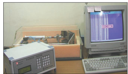
Fig. 5. Cyclic loading system.
