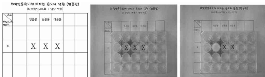
Fig. 5. An developing experiment applying SSC experiment apparatus of precipitate formation for measuring the effect of temperature on chemical reaction rate.
