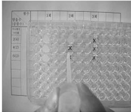
Fig. 2. An developing experiment applying SSC experiment apparatus of precipitate formation for measuring the effect of concentration on chemical reaction rate.
