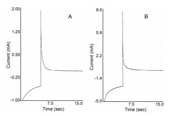
**Figure 1.** Charging current-time profiles of CR (A, graphite powder: CR = 50:50, wt/wt, 6 mm dia.) and glassy carbon electrode (B, 3 mm dia.) in 0.1 M NaCl solution. Step potential; -400 mV,  $t_{\text{max. A}}$ ; 0.201 mA,  $\tau_{\text{A}}$ ; 0.19 sec.,  $t_{\text{max. B}}$ ; 9.0 uA,  $\tau_{\text{B}}$ ; 0.10 sec.
