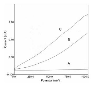
**Figure 2.** LSVs obtained using the carbon powder electrode with CR binder in a stirred 0.1 M NaCl 10 mL at the scan rate of 100 mV/s before (B) and after (C) adding 200  $\mu$ L of 1.0 M H<sub>2</sub>O<sub>2</sub>. A is an LSV of the glassy carbon electrode in 0.02 M hydrogen peroxide solution.
