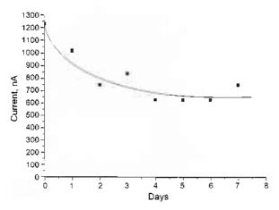
**Figure 5.** Stability determination of the bioelectrode. Sensor response to 0.01 M H<sub>2</sub>O<sub>2</sub> solution was measured over a period of 7 days. Sensor was stored in the air at 4 °C in the dark when not in use.
