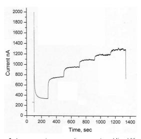
**Figure 3.** Amperometric response for successive adding 100  $\mu$ L of 1.0 M H<sub>2</sub>O<sub>2</sub> in 10 mL of electrolyte solution at -400 mV.
