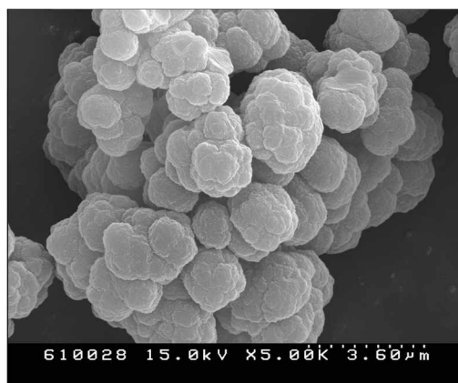
Figure 3. Scanning electron microscope (SEM) image of the imprinted particles.
