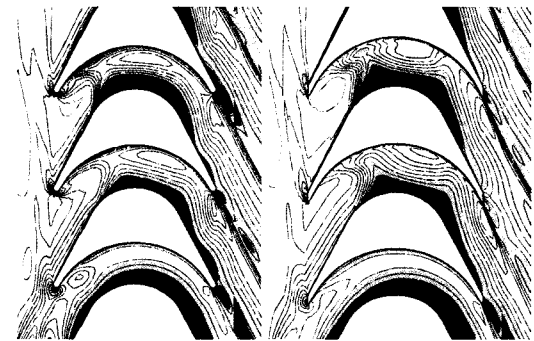
Fig. 9 Iso-Mach Number Contours(10000 rpm)
