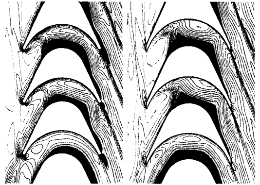
Fig. 8 Iso-Mach Number Contours (0 rpm)
