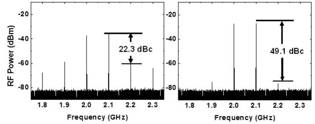
FIG. 9. Measured RF spectra showing the two-tone intermodulation distortions ( $f_1=2.0$  GHz,  $f_2=2.1$  GHz) of the gain-lever DBR laser under (a) free-running and (b) ultra strong injection-locking conditions ( $R=11$  dB,  $\Delta f=-32$  GHz).
