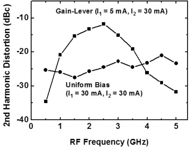
FIG. 6. The second harmonic distortion versus modulation frequency for gain-lever and uniform bias condition. The second harmonic product is measured at twice the RF modulation frequency.
