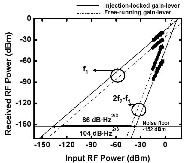
FIG. 10. Measured SFDR of the link with a directly modulated gain-lever DBR laser ( $f_1=2.0$  GHz,  $f_2=2.1$  GHz).
