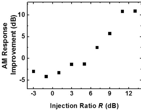
FIG. 8. Measured AM response improvement for various injection ratios. Frequency detuning values are adjusted for the corresponding injection ratios to achieve the largest AM improvement.
