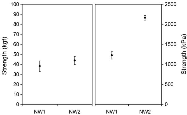
**Figure 5.** Tear (left) and bursting (right) strength.
