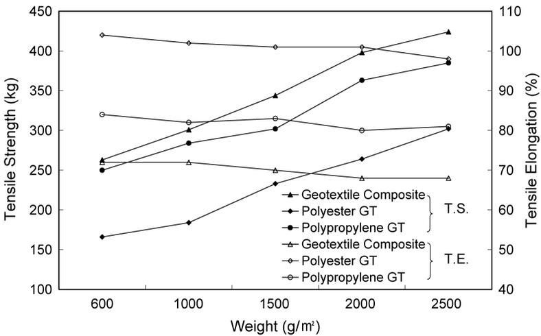
Figure 6. Tensile properties of geotextile composites.
