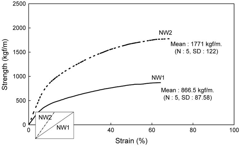
**Figure 4.** Strength–strain curve of geotextile specimen.
