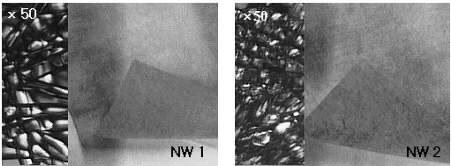
**Figure 3.** Appearance and fiber arrangement of geotextile.
