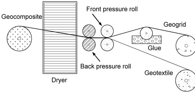
**Figure 1.** Standard manufacturing process for geocomposite.
