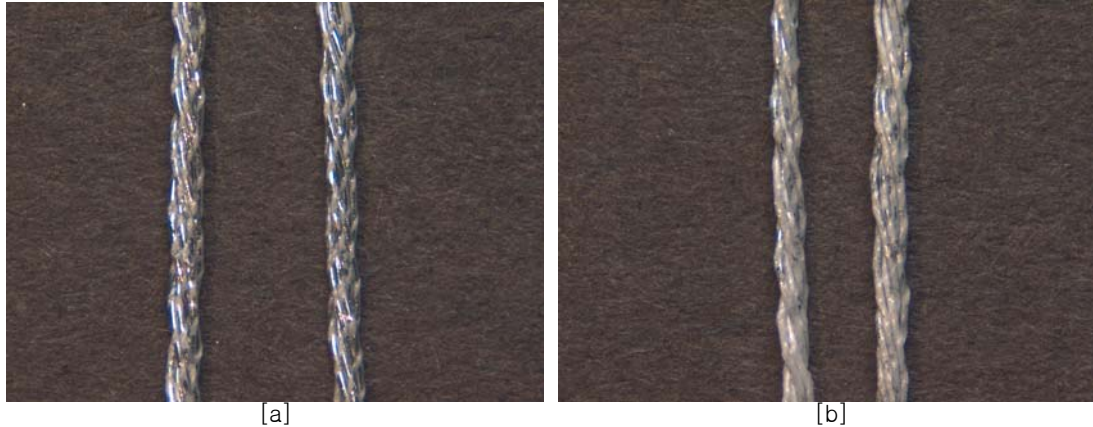
<Fig 8> Change of luster by alkaline treatment, specimen No. 2 (a) 5%, 5min, (b) 5%,10min
