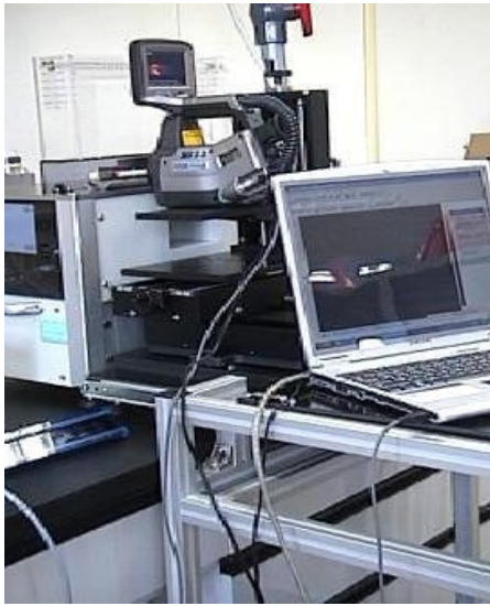
Fig. 1. Experimental setups for measuring the peak temperature of a burning cigarette.
