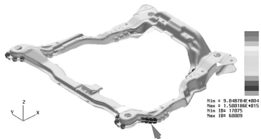
Fig. 7 Fatigue analysis result on the initial model(Model I)
