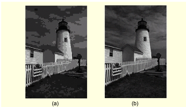
Fig. 7. JPEG distorted images with the PSNR values of (a) 23 dB for gray level and 21dB for EHD, and (b) 28 dB for gray level and 35 dB for EHD.
