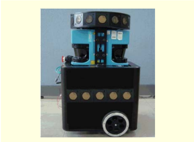
Fig. 12. Mobile robot used for the experiments. This robot has a differential drive type wheel base and is equipped with two laser scanners.
