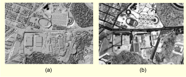
Fig. 2. Visualization of LIDAR coverage: (a) shaded-relief map of range data and (b) intensity image.
