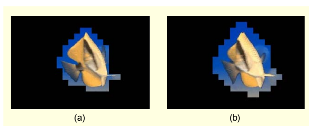
Fig. 9. Obtaining initial OOI: (a) block-based OOI at frame n-1 and (b) OOI expanded at frame n from (a).
