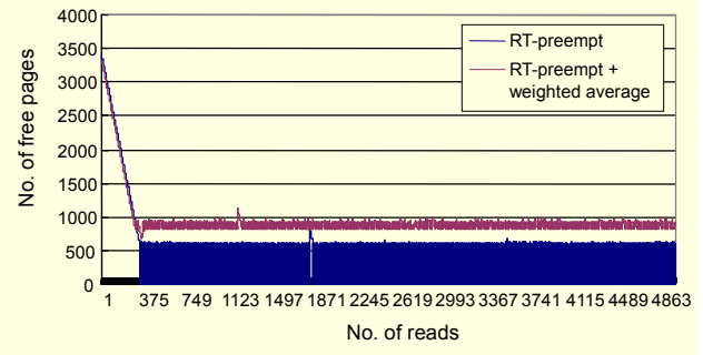
Fig. 15. The number of free pages with and without applying weighted average PIP to kswapd .
