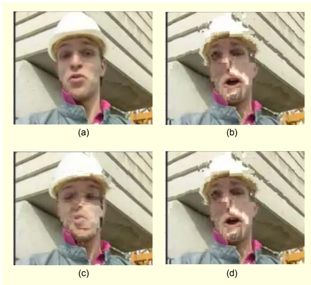
Fig. 12. Frame #92 of the reconstructed Foreman sequence coded at 128 kbps, with frame rate = 10 fps and PLR=10%: (a) error free, (b) redundant slice coded with higher QP, (c) JVT-R058, and (d) redundant slice coded with PD based method.
