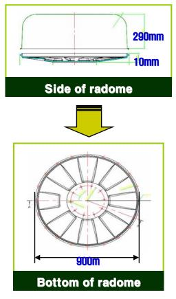
Figure 2. Radome(parabola antenna) standard
