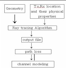
Figure 6. The block diagram for simulation
