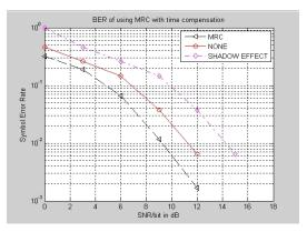
Figure 5. BER for Maximal Ratio Combiner Method (1/2 Blocking)
