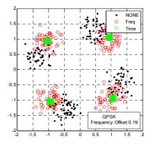
Figure 11. Compensated Constellation (QPSK)
