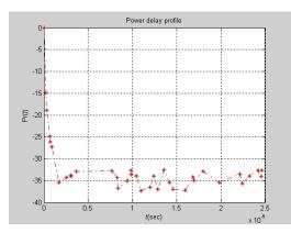
Figure 9. Multipath delay profile
