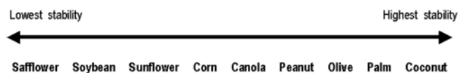
Fig. 4. Relative oxidative stability of some major vegetable oils. Scale is based on inherent oxidative stability, calculated by multiplying the decimal fraction of each unsaturated fatty acid present in a lipid by its relative oxidation rate and then summing these (Erickson and List, 1985).
