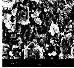
Fig. 6 Micro wick structure(×3,000)
