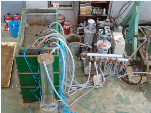
Figure 3. PVD system installation setup.
