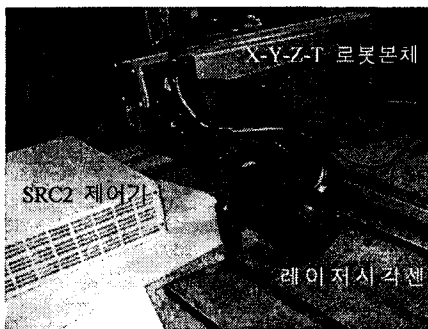
Fig. 13 Seam track test about half V groove
