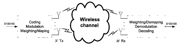
Fig. 4. Diagram of a MIMO wireless transmission system.
