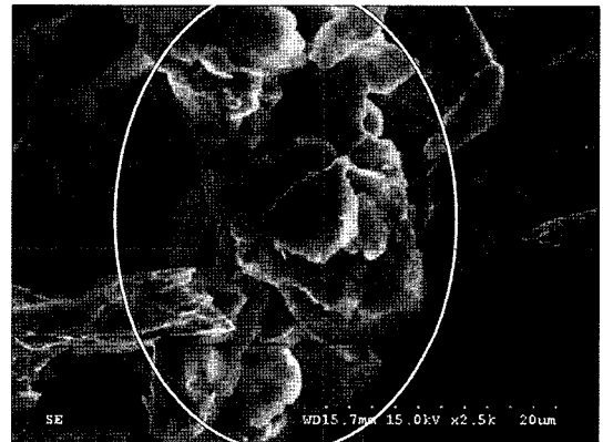
Fig. 9. SEM image of Fe-based powder sheet with 4wt% \text{Al}_2\text{O}_3 powder, showing the agglomerated \text{Al}_2\text{O}_3 particles in a open circle (x2500).
