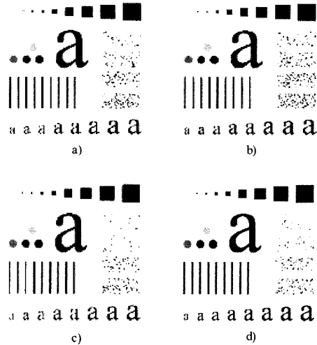
Fig. 9. Interpolation results for 'A alphabet' image by a) Bilinear interpolation, b) Bi-cubic interpolation, c) Triangulation interpolation and d) Proposed adaptive interpolation.
