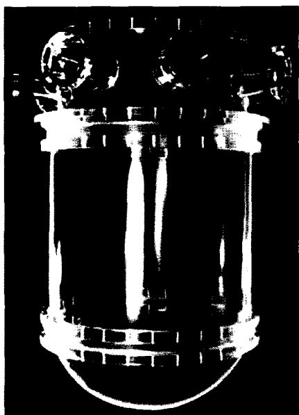
Fig. 1. Reactor Model of the ROCOM Test Facility
