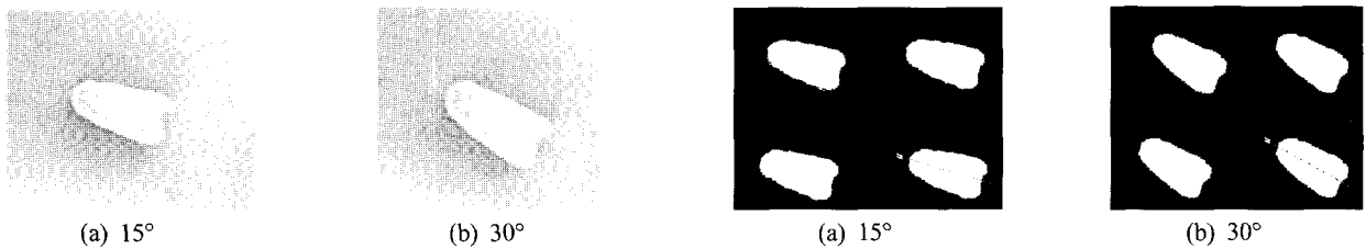
Fig. 16 Input image from CCD camera and results of image processing by the gradient of chambak.
