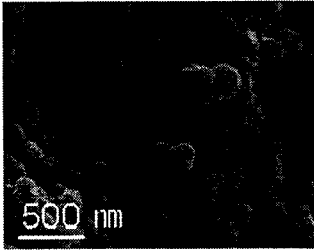
Fig. 3 Morphology of Ni-Zn-ferrite by SEM
