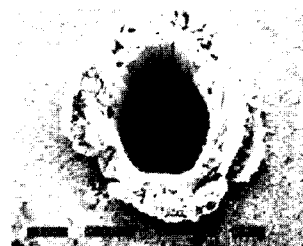
Fig. 2 example of percussion drilling
